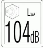
Machines used outdoors are subject to CE marking requirements. Noise emission levels are covered separately. The sample mandatory label shown above specifies noise emission levels.
